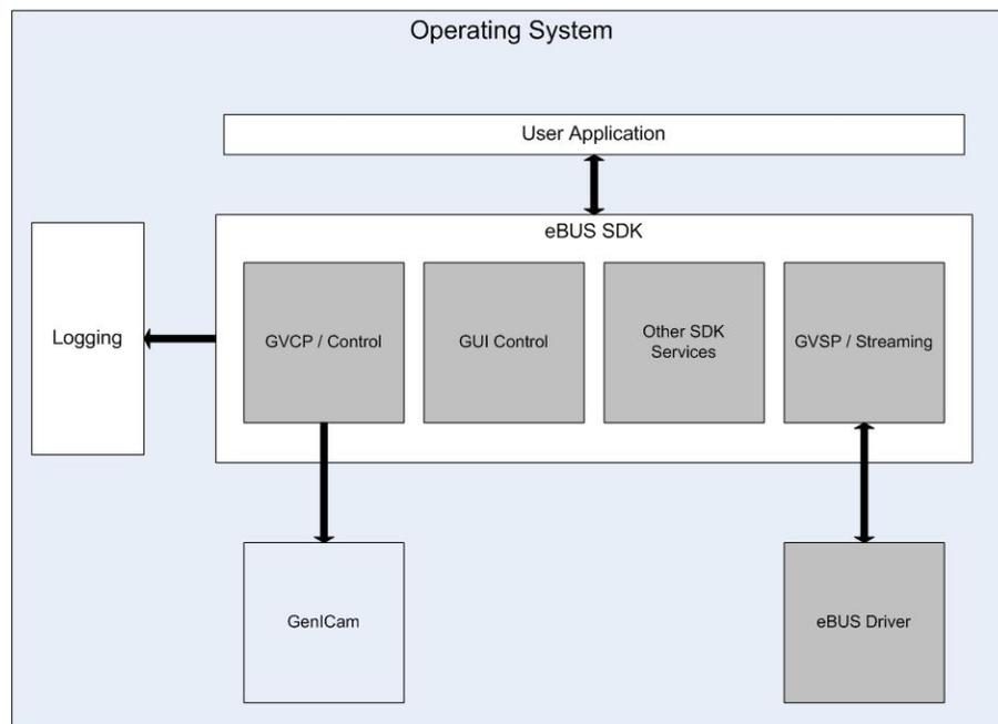
In this example, a user application using the eBUS SDK acts as a receiver that can be used to control and stream video images from the GigE Vision transmitter, for example, a GigE Vision camera. When an application using the eBUS SDK connects to a GigE Vision device, it caches a copy of the XML database to the local memory. Device commands are sent and received through the GVCP command port. Images are received through the GVSP streaming port.
