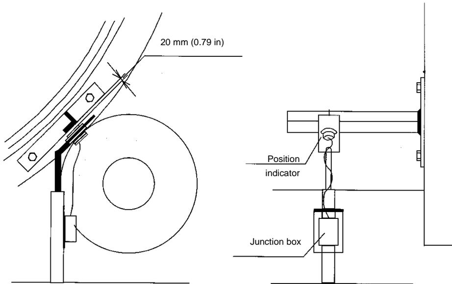
Figure 6-5: Trigger Bar – details –
