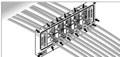
The grommet must produce a continuous seal on the back side.
