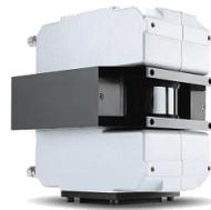
The key component of the CS400 system is the infrared linescanner. The linescanner collects infrared energy, emitted from the kiln surface allowing the system to measure the temperature along the length of the kiln.
