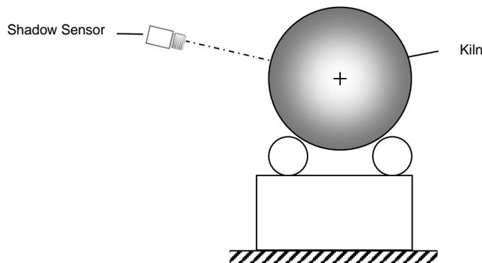
It is important that the sensor is mounted at a distance from the target, sufficient to be able to "see" the entire area of interest. For this reason, the manufacturer provides a field of view calculating software called "Spot Size Calculator", which allows the calculation of the resulting spot size for a given sensor model and based on a specific mounting distance, see <https://www.flukeprocessinstruments.com/SpotSizeCalculator/index.htm>
