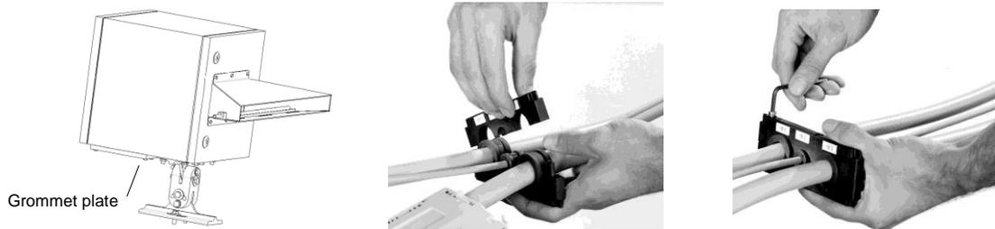
Using the 4 M5x25 screws, mount the grommet plate on the outside of the protective housing. Plug the cable connectors into the linescanner. Connect the socket and the plug for earth ground.
