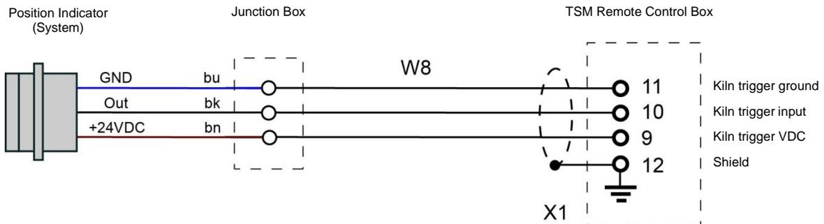
Figure 8-9: Terminal Wiring for the Position Indicator (Ring 1)
