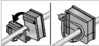
Lay cable into appropriate grommet and provide strain relief where necessary using cable ties.
