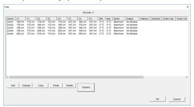
You can adjust them further by double clicking on the zones. The mode selection represents how the zone temperature will be displayed/saved (e.g. max, average, minimum, etc)
