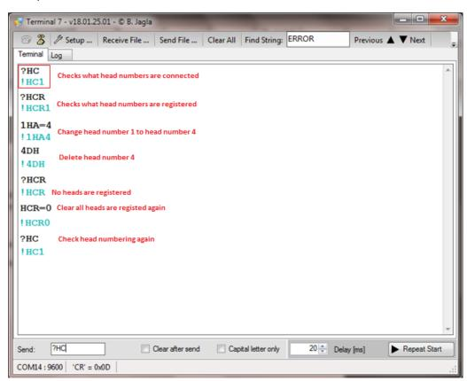
In case of replacing a given head, ensure to use the **DH** command after removing the old head and before replacing the new head. Double check using the **?HCR** command. In case you have not deleted the head number before replacement, use *n"old number"*HA=*n"new number"* to change the head number after using the DH command.
