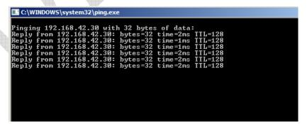
Note: The first three octets of IP address of PC should be same as that of scanner i.e. for the example given above the IP address of the PC can be 192.168.42.X (where X can be any digit from 0 to 255 except 30)
