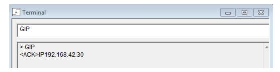
Step 9-Next you will type in the new IP address that you want the connected scanner to be. I will be using 192.168.42.31. Clear out GIP in the command window and enter IP192.168.42.31. A few seconds after you change the IP address there will be a popup error-Timeout after sending command! Select OK and close the ES150 software
