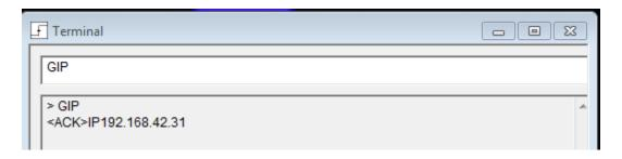
Step 16-Clear GIP in the command window and enter PS, to save the new Parameter. Your response will be a PS and <ACK>
